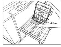
To close the lower guide plate, hold its handle with your right hand and lift the lever up to unlatch it with your left hand. Then put it down slowly.
